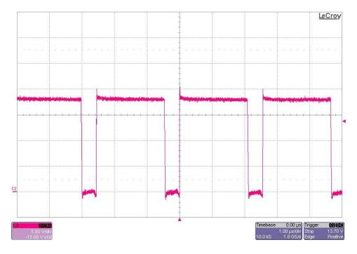
The photo below shows the switch node measured with 200MHZ bandwidth. The input voltage is 24V and the output is loaded to 1A. (5V/DIV, 1uS/DIV)
