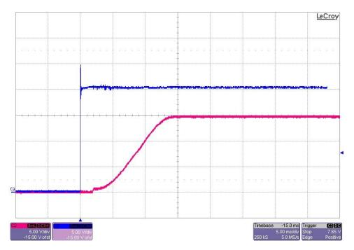
The photo below shows the output voltage startup waveforms after the application of 20V in. The 15V output was loaded to 5A. (5V/DIV, 5mS/DIV)
