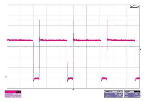
The photo below shows the switch node measured with 200MHZ bandwidth. The input voltage is 24V and the output is loaded to 5A. (5V/DIV, 1uS/DIV)
