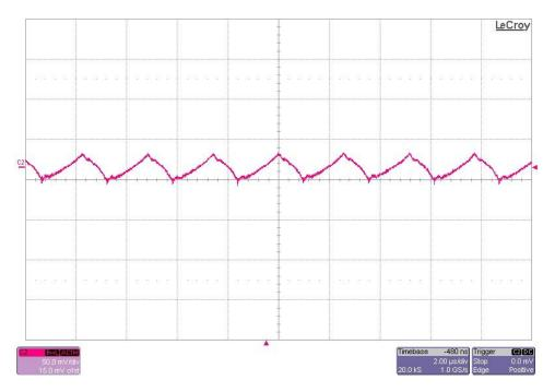
The output ripple voltage is shown in the figure below. The image was taken with the 15V output loaded to 5A. The input voltage set to 18V. (50mV/DIV, 2uS/DIV)
