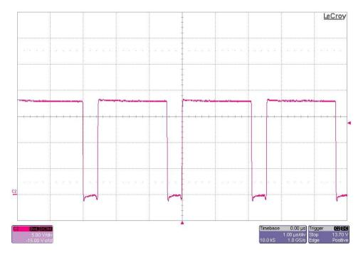
The photo below shows the switch node measured with 20MHZ bandwidth. The input voltage is 24V and the output is loaded to 5A. (5V/DIV, 1uS/DIV)
