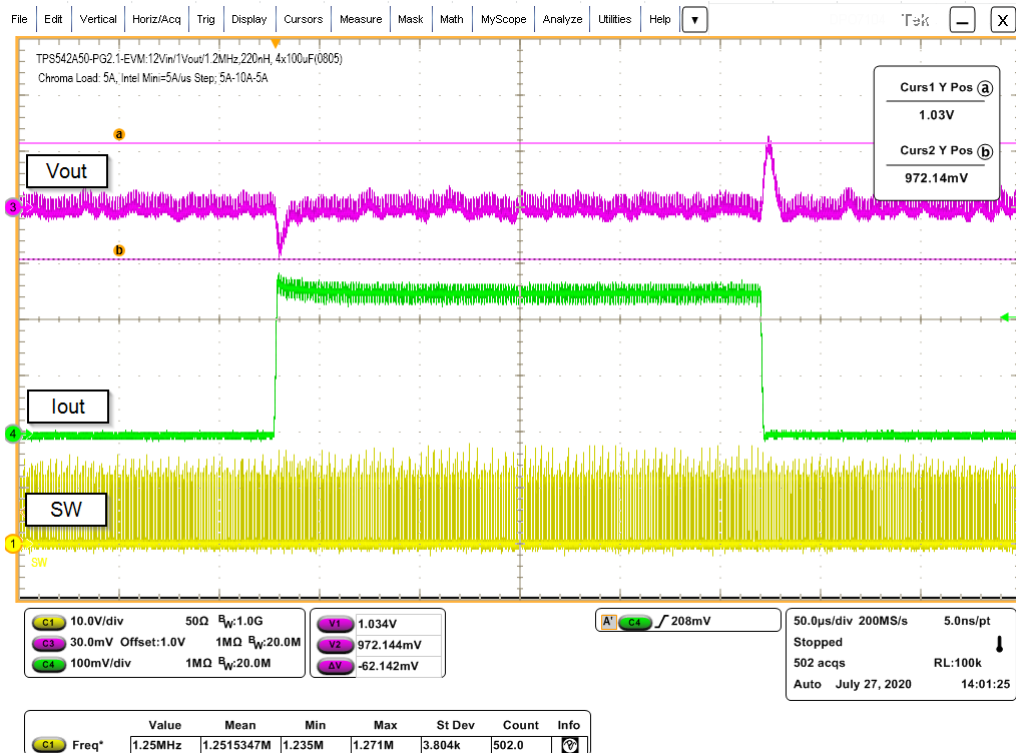
Figure 4-6. Transient response - 5-A to 10-A to 5-A load @5 A/ \mu s, \Delta V_{out} = 62.1 mV, f_{sw} = 1200 kHz, FCCM
