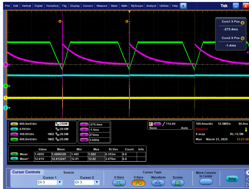
Figure 3-12. Steady State Waveforms at 0 A (Ch1= ISNS; Ch2 = Vout; Ch3 = SW; Ch4 = I_OPT)
