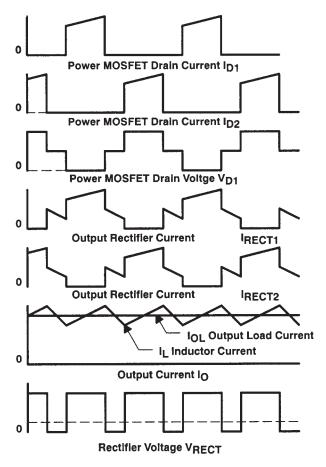
Figure 18. Push-Pull Converter Waveforms
