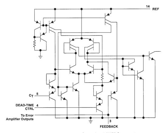
Figure 8. Dead-Time-Control and PWM Comparator
