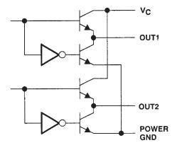
Figure 16. Totem-Pole Output Circuits
