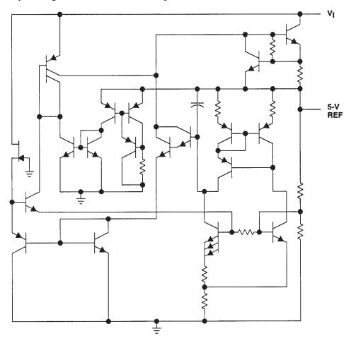
Figure 3. 5-V Reference Regulator Schematic
