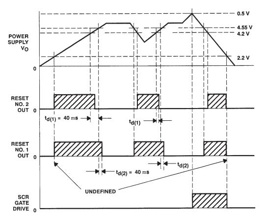
Figure 27. Overvoltage/Undervoltage Circuits Timing Diagram
