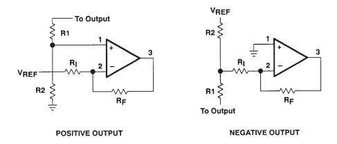
Figure 11. Error Amplifier Bias Circuits for Controlled Gain Applications
