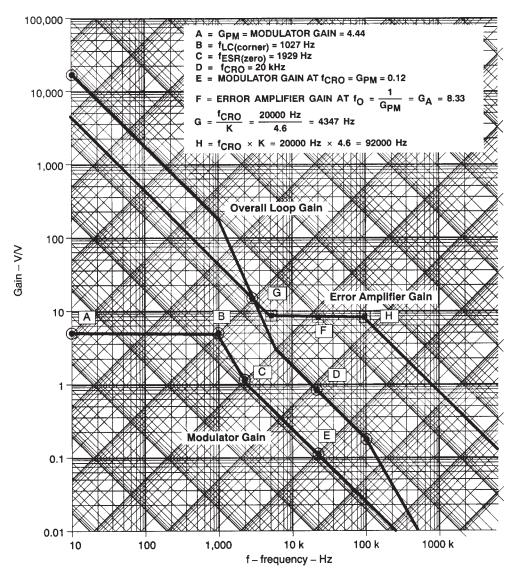
Figure 24. Power Modulator/Output Filter Gain vs Frequency
