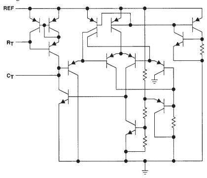
Figure 5. Oscillator Schematic
