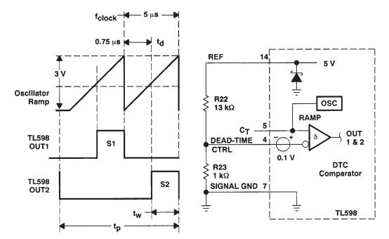
Figure 19. DTC Comparator Circuit and Waveforms
