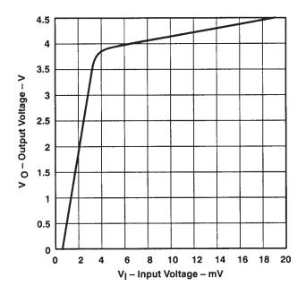
Figure 12. Amplifier Transfer Characteristics
