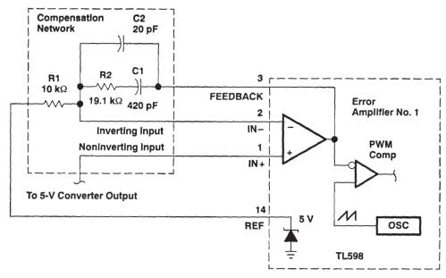
Figure 25. Error Amplifier and Loop Compensation Circuits
