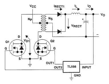
Figure 17. Push-Pull Converter Power Section
