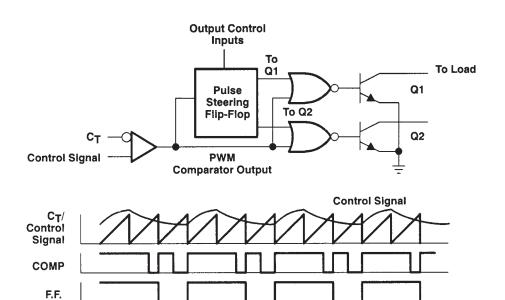
Figure 14. Output Steering Circuit
