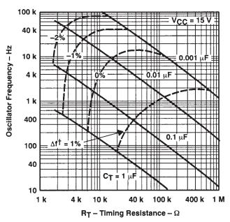
$<sup>^{\</sup>dagger}$  Frequency variation ( $\Delta f$ ) is the change in oscillator frequency that occurs over the full temperature range.
