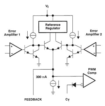
Figure 10. MUX Structure of Amplifiers
