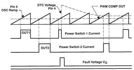
Figure 21. Overcurrent Protection Circuit and Waveforms
