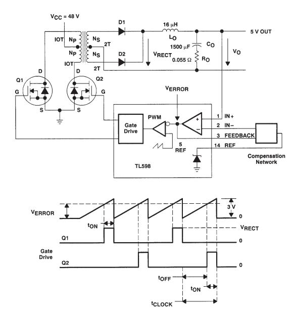
Figure 23. Error Amplifier and Compensation Circuits With Waveforms
