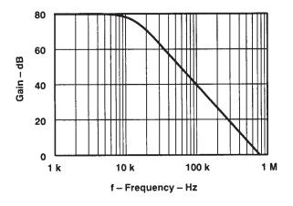
Figure 13. Amplifier Bode Plot
