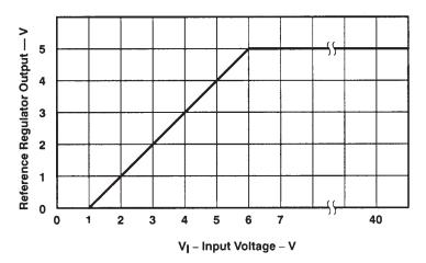
Figure 4. 5-V Reference Regulator Output vs Input Voltage
