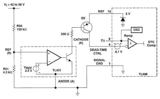
Figure 22. Overvoltage Protection Circuit
