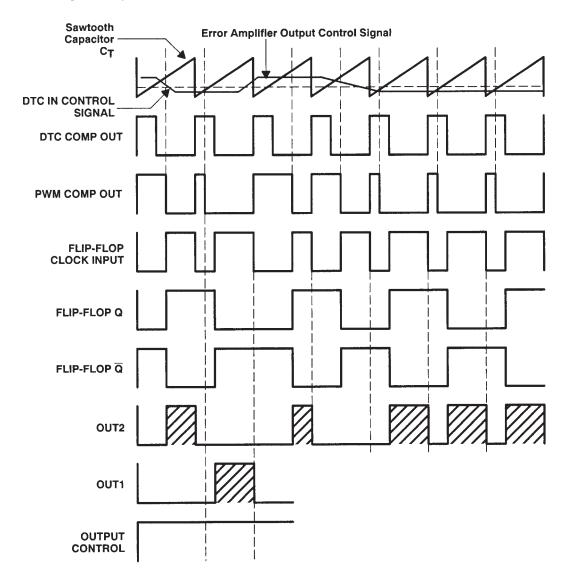
Figure 2. TL598 Circuit Timing Waveforms
