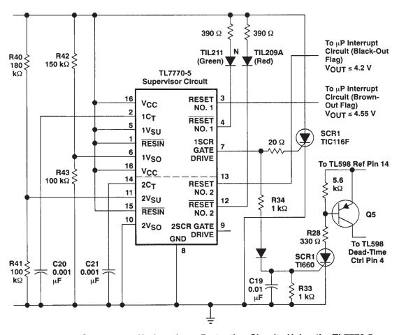
Figure 26. Overvoltage/Undervoltage Protection Circuits Using the TL7770-5
