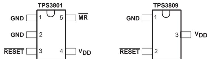
**Figure 3. Terminal Assignment**
