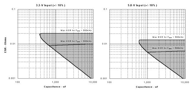
Figure 3. Regions of Stability for 2.2- $\mu\text{H}$  Inductor
