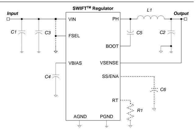
Figure 1. Typical Schematic
