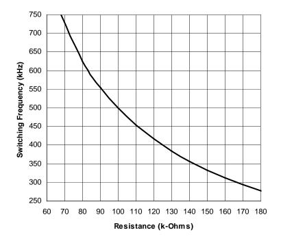
Figure 2. Switching Frequency Trimming Resistor Selection
