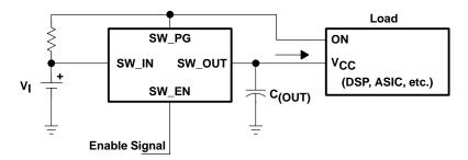
Figure 8. Power Large Load Through Power Sequencing
