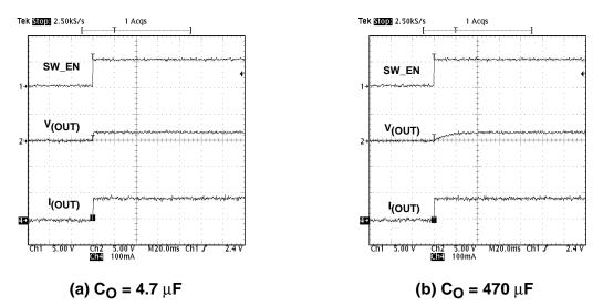
Figure 7. Power Switch Power-Up With 20- $\Omega$  DC Load
