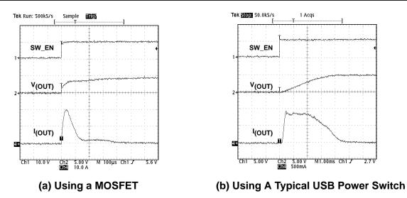
Figure 1. Inrush Current During Power on With a 470-µF Capacitive Load
