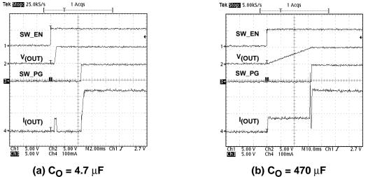
Figure 9. Powering Large-Current Load With TPS2150/51
