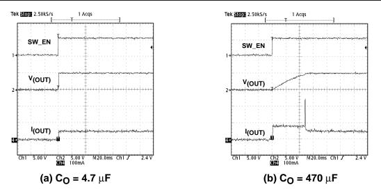
Figure 5. Power Switch Power-Up With Small DC Load (R<sub>L</sub> = 100  $\Omega$ )
