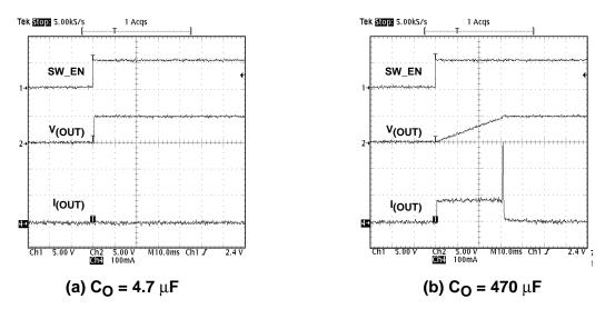
Figure 3. Power Switch Power-Up Into a Pure Capacitive Load
