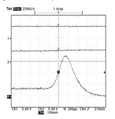
Figure 4. Power Switch Power-Up Into a Pure Capacitive Load (*Zoomed-in* View of Figure 3(b))
