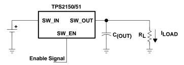
Figure 2. Simple Application Diagram for Power Switch
