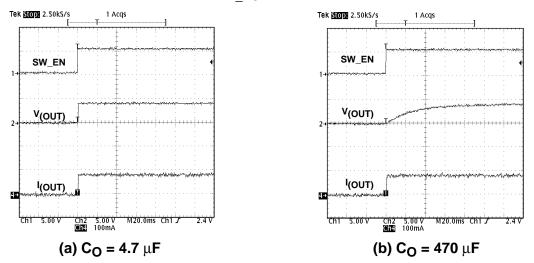
Figure 6. Power Switch Power-Up With 50- $\Omega$  DC Load
