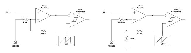
Figure 1. Feedback Section of the TPS54x11, TPS54x12 and TPS54x13
