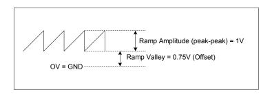
Figure 3. Ramp Waveform
