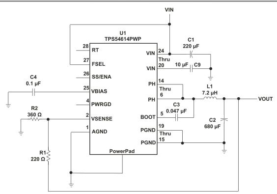
Figure 6. TPS54614 Schematic Adjusted for VOUT = 2.9 V
