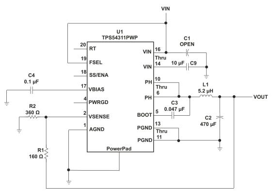
Figure 8. TPS54311 Schematic Adjusted for VOUT = 1.3 V
