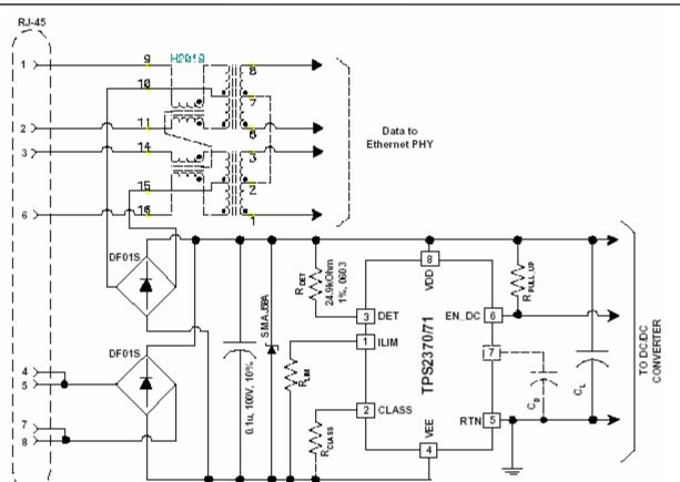
Figure 2. A Typical PD Front-End Application Diagram With TPS2370/71
