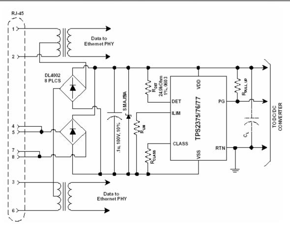
Figure 3. A Typical PD Front-End Application Diagram With TPS2375/77
