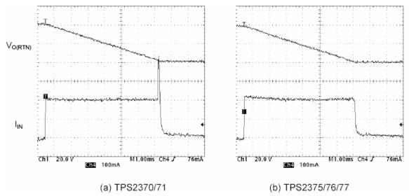
Figure 1. Inrush Current Limit and Termination Comparison of PDCs
