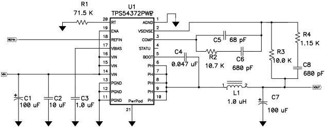
Figure 1. Typical TPS54372 Application Circuit
