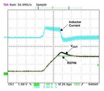
Figure 2. REFIN Rising-Edge Slew Rate at Maximum
