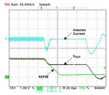
Figure 6. REFIN Falling-Edge Slew Rate Above Maximum
