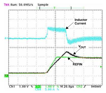
Figure 3. REFIN Rising-Edge Slew Rate Above Maximum
