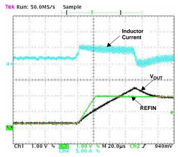
Figure 4. REFIN Rising Edge with 2-A Output Current
