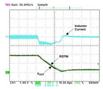
Figure 5. REFIN Falling-Edge Slew Rate at Maximum
