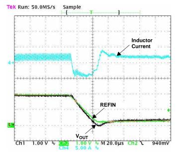
Figure 7. REFIN Falling Edge with 2-A Output Current
