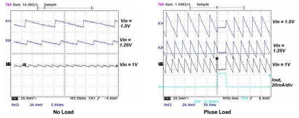
Figure 7. Output Ripple Voltage During PFM-Mode Operation With 10- $\mu$ H Inductance, 2 × 4.7- $\mu$ F + Additional 22- $\mu$ F (C5) Output Capacitor
