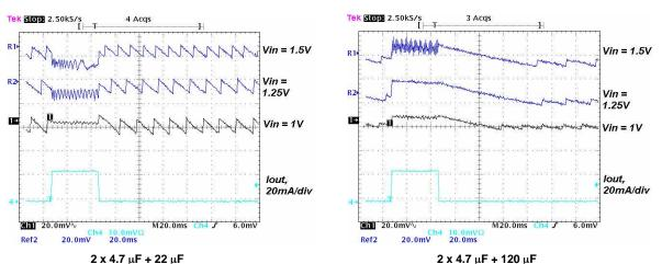
Figure 11. Output Ripple Voltage During PFM-Mode Operation With 1-nF Feedforward Capacitor (Cff), 4.7-µH Inductor, and With Different Output Capacitors
