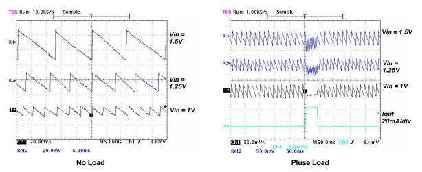
Figure 3. Output Ripple Voltage During PFM-Mode Operation With Original EVM Setup of 4.7- $\mu$ H Inductor and 2 × 4.7- $\mu$ F Output Capacitors (Note the change of voltage scale on the right to accommodate the waveforms.)
