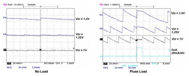
Figure 5. Output Ripple Voltage During PFM-Mode Operation With Additional 120-µF Output Capacitor (C5)
