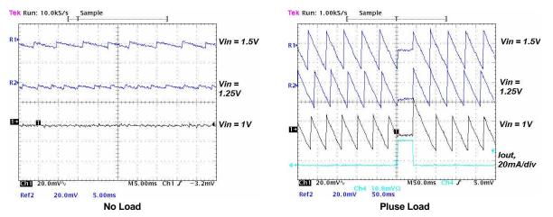
Figure 9. Output Ripple Voltage During PFM-Mode Operation With 22- $\mu$ H Inductance, 2 × 4.7- $\mu$ F + 22- $\mu$ F (C5) Output Capacitor
