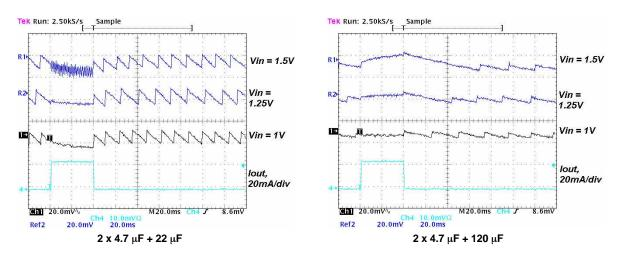
Figure 16. Output Ripple Voltage During PFM-Mode Operation With 100-nF Feedforward Capacitor (Cff), 10-µH Inductor, and With Different Output Capacitors
