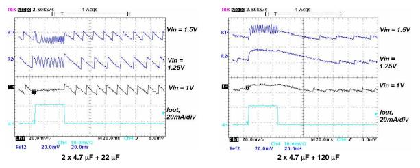
Figure 12. Output Ripple Voltage During PFM-Mode Operation With 10-nF Feedforward Capacitor (Cff), 4.7-µH Inductor, and With Different Output Capacitors
