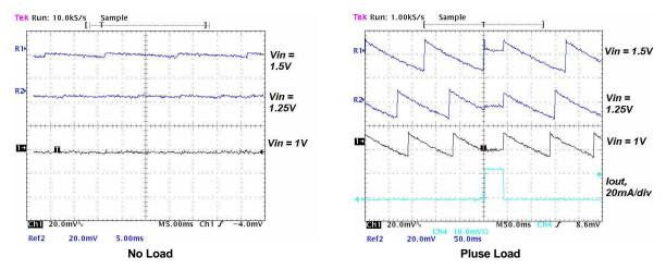
Figure 8. Output Ripple Voltage During PFM-Mode Operation With 10- $\mu$ H Inductance, 2 × 4.7- $\mu$ F + Additional 120- $\mu$ F(C5) Output Capacitor
