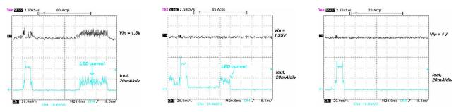
Figure 20. Output Ripple Voltage and Current Waveform From TPS61070 During Sniff-Mode Operation of Bluetooth Headset With 1-nF Feedforward Capacitor (Cff) and With  $2 \times 22$ -µF Output Capacitors
