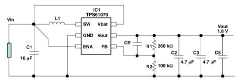
Figure 2. Test Circuit of TPS61070 for Single-Cell Alkaline Battery to 1.8-V Output
