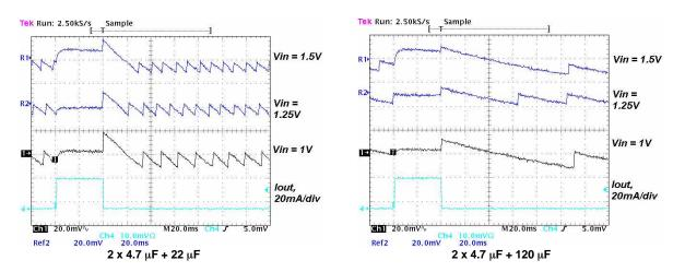
Figure 18. Output Ripple Voltage During PFM-Mode Operation With 10-nF Feedforward Capacitor (Cff), 22-µH Inductor, and With Different Output Capacitors
