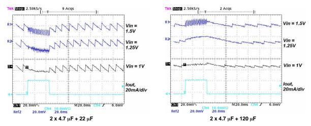
Figure 13. Output Ripple Voltage During PFM-Mode Operation With 100-nF Feedforward Capacitor (Cff), 4.7-µH Inductor, and With Different Output Capacitors
