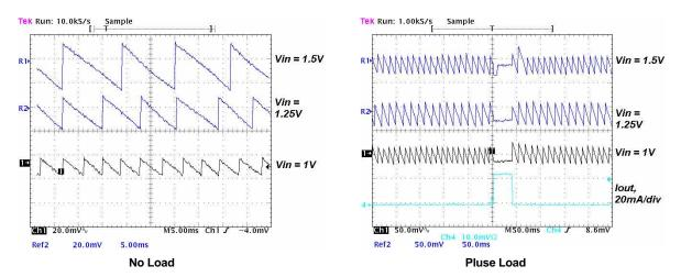
Figure 6. Output Ripple Voltage During PFM-Mode Operation With 10-µH Inductance, 2 × 4.7-µF Output Capacitor (Note the change of voltage scale on the right to accommodate the waveforms.)
