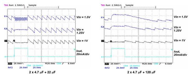
Figure 15. Output Ripple Voltage During PFM-Mode Operation With 10-nF Feedforward Capacitor (Cff), 10-µH Inductor, and With Different Output Capacitors
