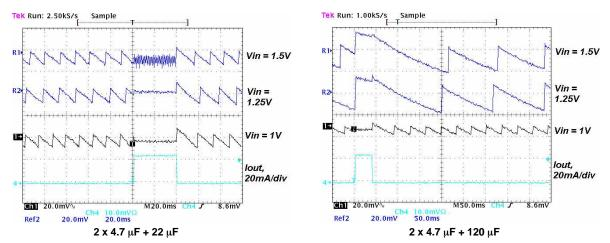
Figure 14. Output Ripple Voltage During PFM-Mode Operation With 1-nF Feedforward Capacitor (Cff), 10µH Inductor, and With Different Output Capacitors
