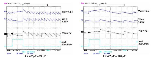
Figure 19. Output Ripple Voltage During PFM-Mode Operation With 100-nF Feedforward Capacitor (Cff), 22-µH Inductor, and With Different Output Capacitors
