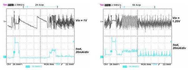
Figure 1. High Ripple Voltage Causes the Bluetooth Chipset to Draw Excessive Current During Sniff-Mode Operation
