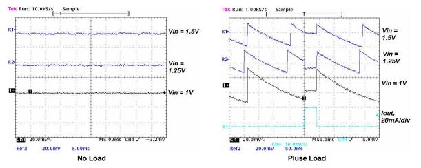
Figure 10. Output Ripple Voltage During PFM-Mode Operation With 22- $\mu$ H Inductance, 2 × 4.7- $\mu$ F + 120- $\mu$ F (C5) Output Capacitor
