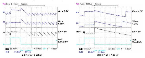
Figure 17. Output Ripple Voltage During PFM-Mode Operation With 1-nF Feedforward Capacitor (Cff), 22µH Inductor, and With Different Output Capacitors
