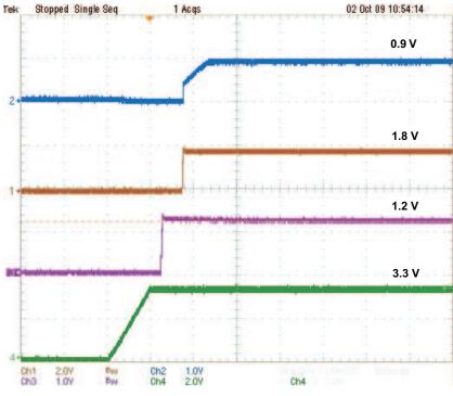
Figure 2. Power-Up Waveform, Part 1
