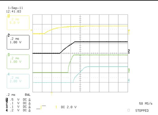
Figure 3. TPS650061 Power-On Ch1-Vin, Ch2-VODC, Ch3-VLDO2, Ch4-VLDO1
