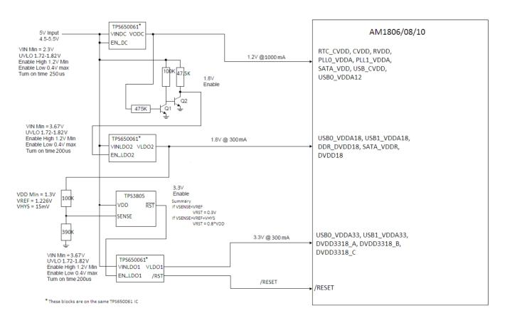
Figure 1. TPS3805, TPS650061, and AM1806/08/10 Block Diagram
