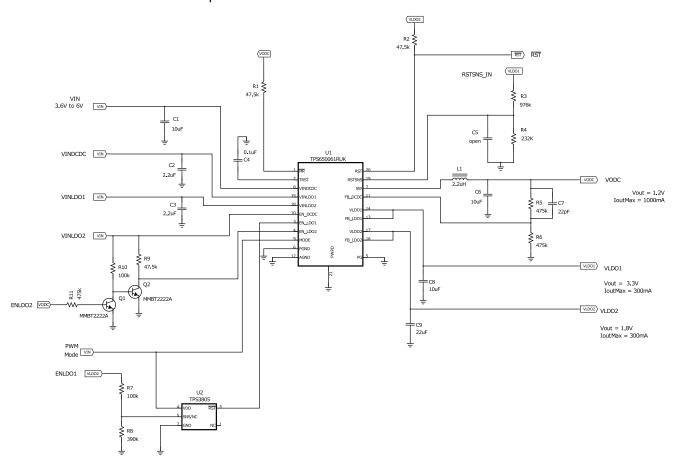
Figure 2. TPS650061 Schematic Diagram
