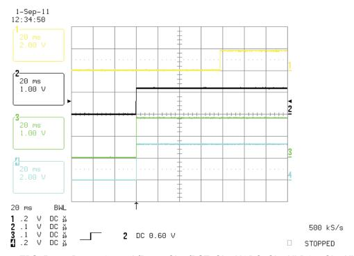
Figure 4. TPS650061 Power-On and /Reset Ch1-/RST, Ch2-VODC, Ch3-VLDO2, Ch4-VLDO1
