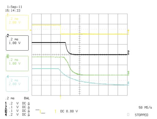
Figure 5. TPS650061 Power-Off Ch1-/RST, Ch2-VODC, Ch3-VLDO2, Ch4-VLDO1
