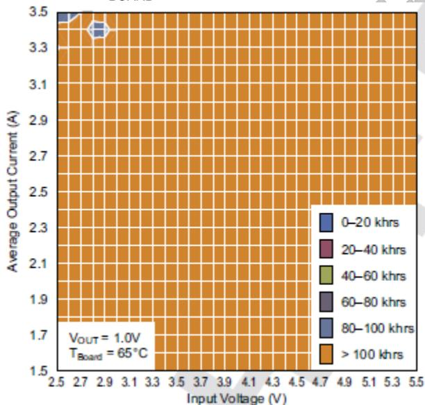
Figure 1. Lifetime for  $V_{OUT} = 1.0\text{ V}$ ,  $T_{BOARD} = 65^{\circ}\text{C}$
