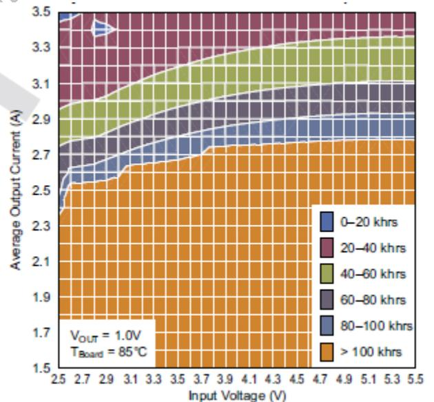
Figure 2. Lifetime for  $V_{OUT} = 1.0\text{ V}$ ,  $T_{BOARD} = 85^{\circ}\text{C}$
