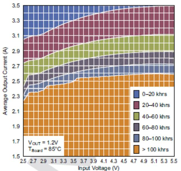
Figure 4. Lifetime for  $V_{OUT} = 1.2\text{ V}$ ,  $T_{BOARD} = 85^\circ\text{C}$
