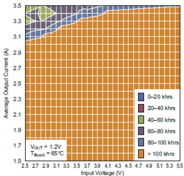
Figure 3. Lifetime for  $V_{OUT} = 1.2\text{ V}$ ,  $T_{BOARD} = 65^\circ\text{C}$
