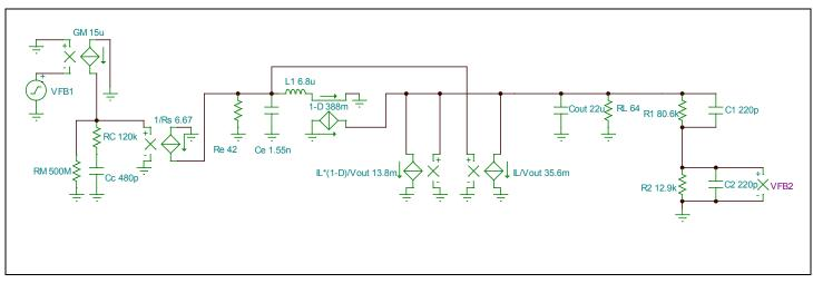
**Figure 7.** Loop Compensation With the Two External Capacitors C1 and C2 By the simulation, the Bode plot can be obtained in Figure 8.
