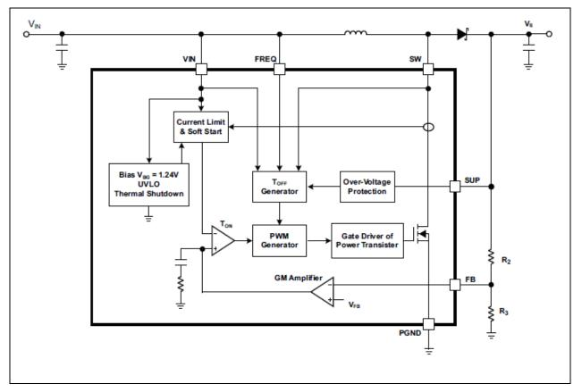
Figure 1. TPS65142 Boost Converter Implementation
