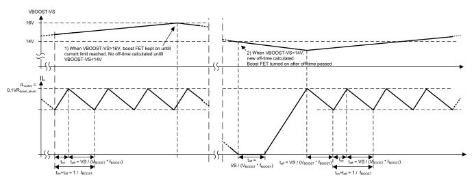
Figure 2. Boost Waveforms Showing Burst Pulsing Controlled by Hysteretic Comparator Levels
