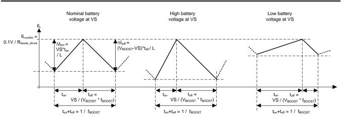
Figure 1. Coil Current Waveforms in Steady State for Nominal, High and Low Battery Voltage
