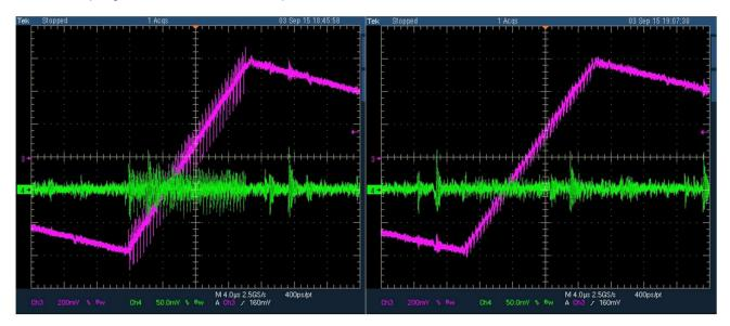
Figure 4. Boost Output and Current Sense O1 Output, Before and After Bypass Capacitor
