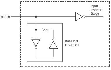
Figure 7. Typical Bus-Hold Cell
