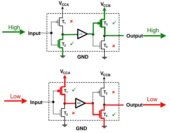
Figure 1. Basic Operation of LVC Devices
