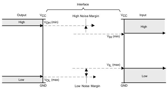
Figure 2. Logic Compatibility Between I/Os
