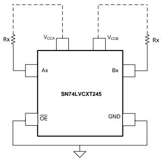
Figure 9. Pull-up Resistors on Inputs
