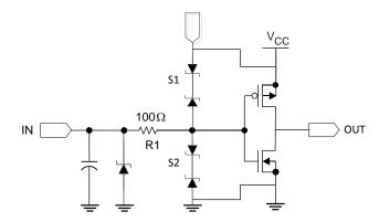
Figure 4. CMOS Input Circuits With ESD Diodes
