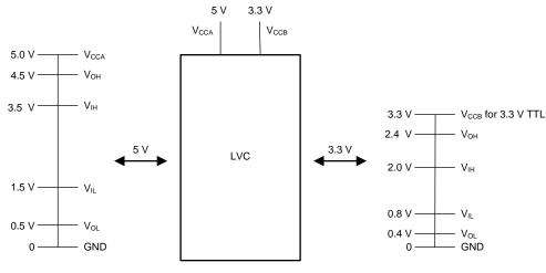
5 V CMOS Device I/O Levels
