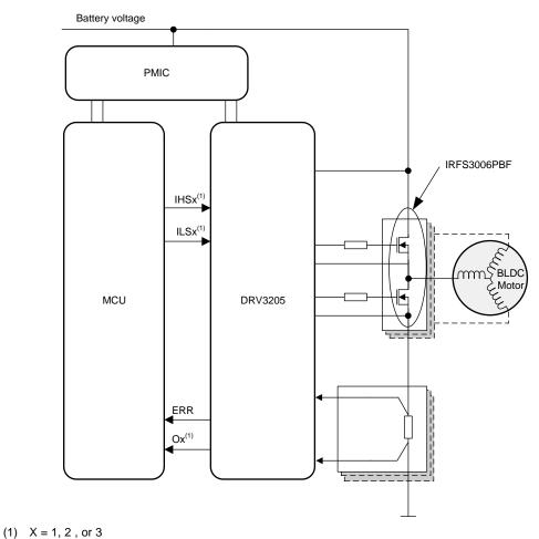
Figure 1. Test Schematic
