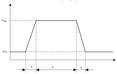
Figure 2. Supply Profile 1 Timing Chart
