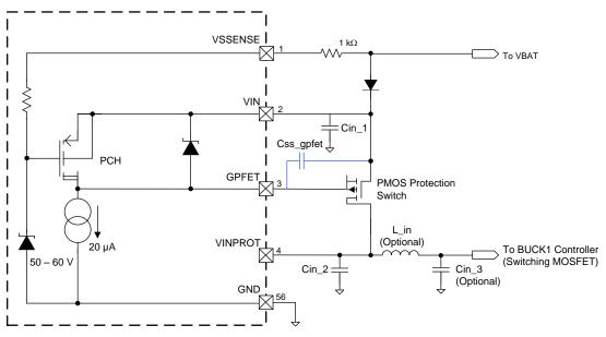
Figure 1. GPFET PMOS Switch Drive Control Circuitry With Css\_gpfet
