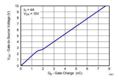
Figure 2. MOSFET Gate Charge
