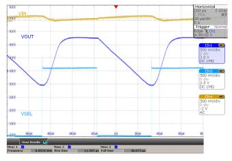
Figure 3. VSEL toggled with 10kHz,  $V_1 = 5 V$ ,  $V_0 = 3.3 V$  or 5V, forced-PWM
