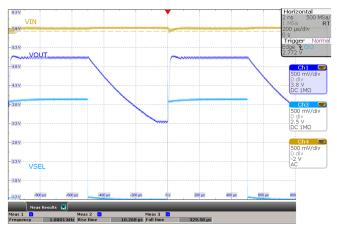
Figure 6. Power save mode. V<sub>I</sub>= 5V, V<sub>O</sub>= 3.3 V or 5 V, I<sub>O</sub>= 125 mA, PSM
