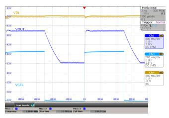
Figure 5. Power save mode. V<sub>I</sub>= 5 V, V<sub>o</sub> = 3.3 V or 5 V, I<sub>o</sub> = 250 mA, PSM
