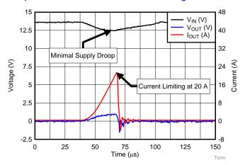
Figure 4. Short Circuit Waveform (Adjustable I<sub>LIM</sub>)
