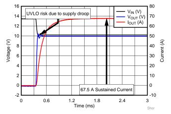
Figure 3. Short Circuit Waveform (Fixed High ILIM)
