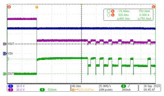
Figure 3. Waveform of the TPS27S100 During an Overload Condition (5-Ω / 4.2-A Load)
