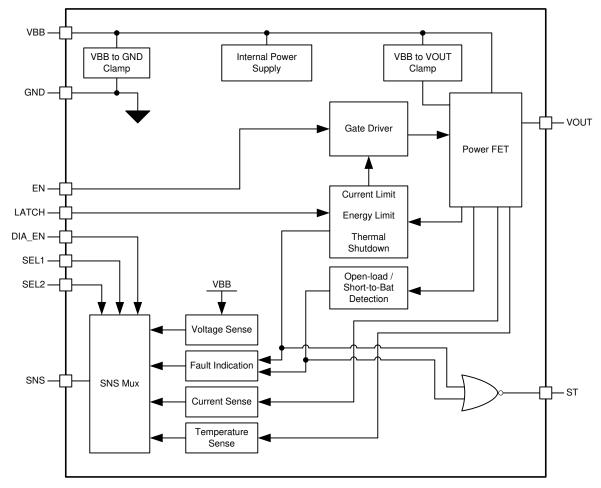
Figure 1-1. Functional Block Diagram
