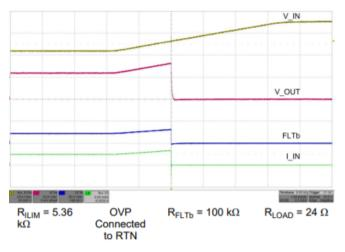
Figure 4. TPS26600 Over Voltage Cut-off Response
