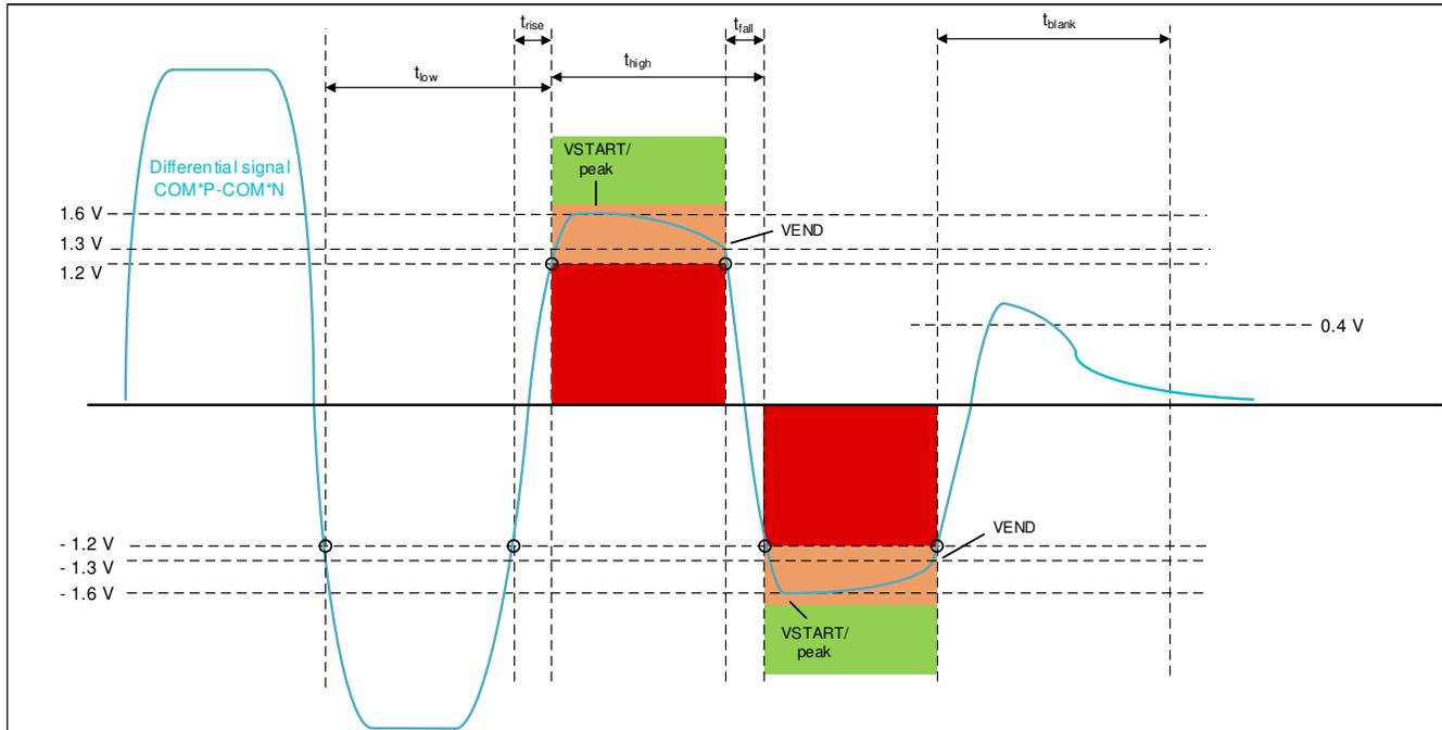
**Figure 3-2. Differential Signal Eye Diagram - 1.6 V VSTART**
