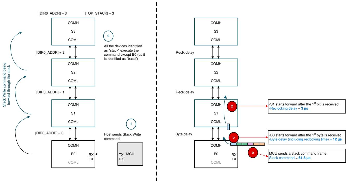
Figure 6-2. How a Stack Command is Sent
