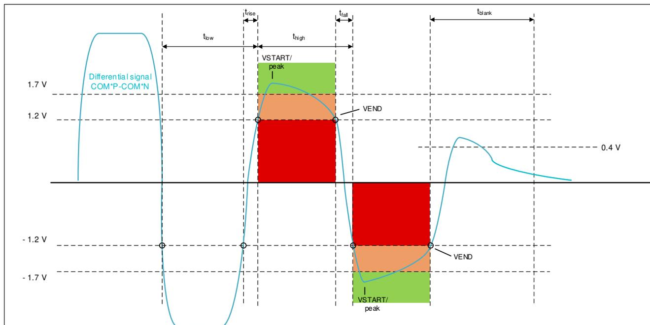
Figure 3-1. Differential Signal Eye Diagram - 1.7 V VSTART
