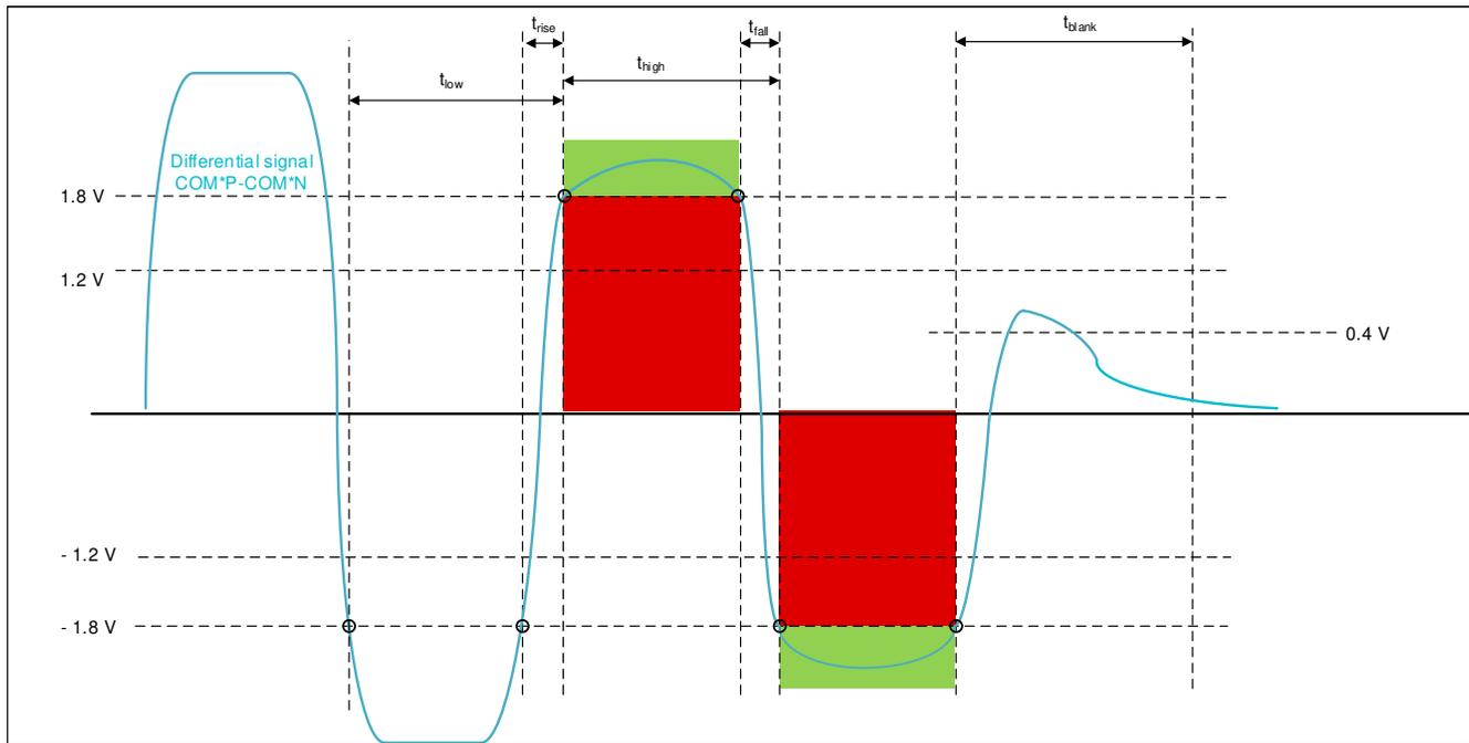
Figure 3-3. Differential Signal Eye Diagram - BQ79600
