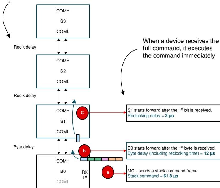
The timing analysis can be different depends on the definition of start and stop of time count
