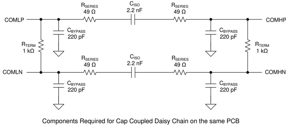
Figure 5-3. Capacitor Only on Same PCB
