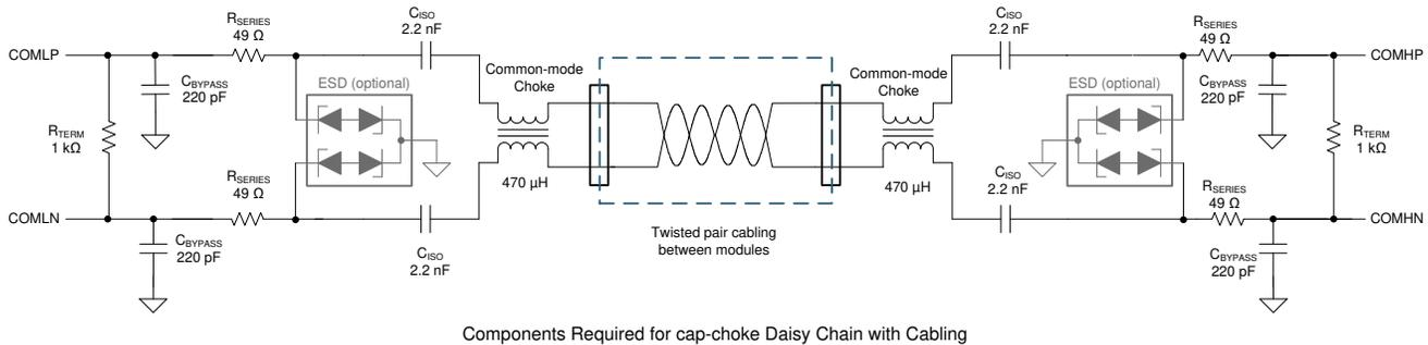
Figure 5-4. Capacitor and Choke Across PCBs
