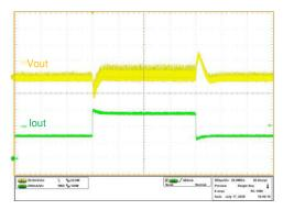
Figure 4-3. Load Transient -  $V_{IN}$  = 0.7 V,  $V_{OUT}$  = 3.3 V,  $I_{OUT}$  = 0.3 A to 0.6 A
