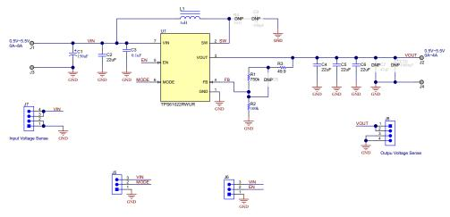
Figure 1-1. TPS61022 EVM Schematic
