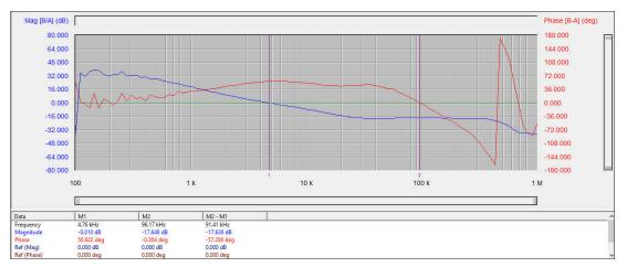
Figure 4-5. Bode Plot -  $V_{IN}$  = 0.7 V,  $V_{OUT}$  = 3.3V,  $I_{OUT}$  = 0.6 A
