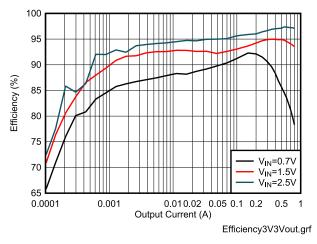
Figure 4-7. Load Efficiency With Different Input in Auto PFM
