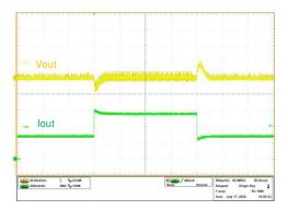
Figure 4-4. Load Transient -  $V_{IN}$  = 1.5 V,  $V_{OUT}$  = 3.3 V,  $I_{OUT}$  = 0.3 A to 0.6 A
