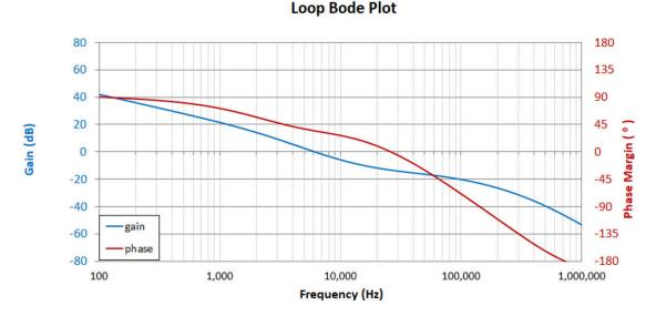
Figure 3-1. Bode Plot in  $V_{IN}$  = 0.7 V,  $V_{OUT}$  = 3.3 V,  $I_{OUT}$  = 0.8 A,  $C_{OUT}$ = 30 µF Condition
