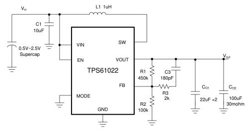
Figure 4-1. TPS61022 Circuit With Feedfoward Capacitor
