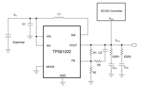
Figure 2-1. TPS61022 Boost Converter in Supercap Backup Power Applications
