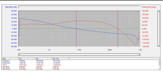
Figure 4-6. Bode Plot -  $V_{IN}$  = 1.5 V,  $V_{OUT}$  = 3.3 V,  $I_{OUT}$  = 0.6 A
