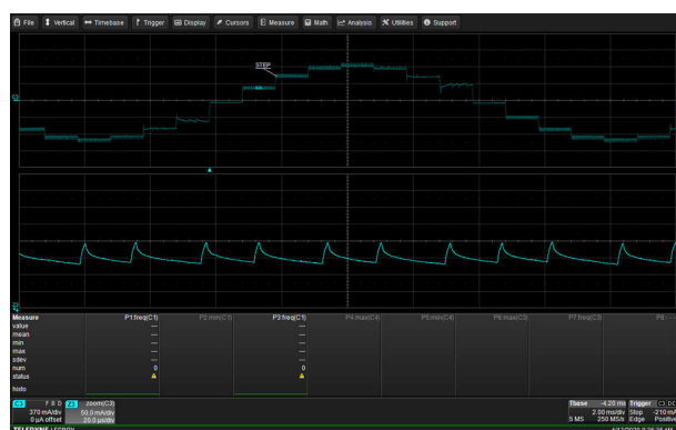
Figure 3-12. PWM at 38% Level, PWM Frequency is 55kHz
