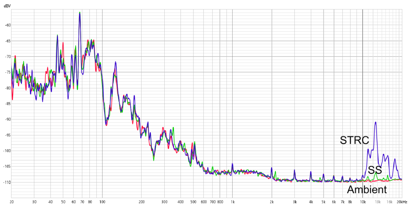
Figure 3-11. Silent Step Decay Mode (SS) vs Smart Tune Ripple Control (STRC) at 1/256 Microstepping
