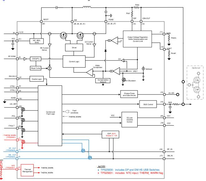
Figure 1-1. Functional Block Diagram
