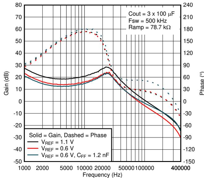
Figure 5-3. Bode plot with lower reference voltage and feedforward capacitor (12-V input, 1.8-V output, 20-A load)
