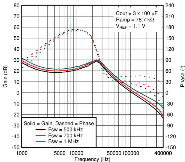
Figure 4-1. Bode plot for different switching frequency (12-V input, 1.8-V output)
