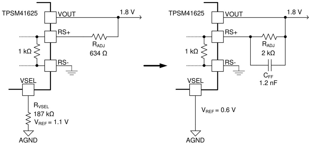
Figure 5-2. Changes to lower reference voltage and add feedforward capacitor
