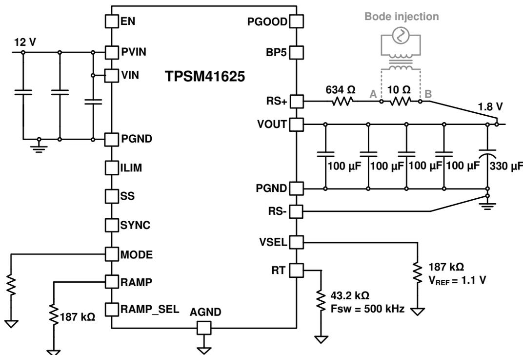
Figure 1-1. Original 12-V input, 1.8-V output, 25-A, 500-kHz design
