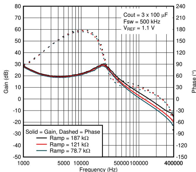
**Figure 3-2. Bode plot for different ramp setting (12-V input, 1.8-V output)**
