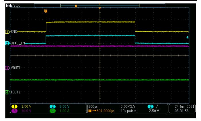
Figure 2-3. Current Sense with DIAG\_EN Toggling
