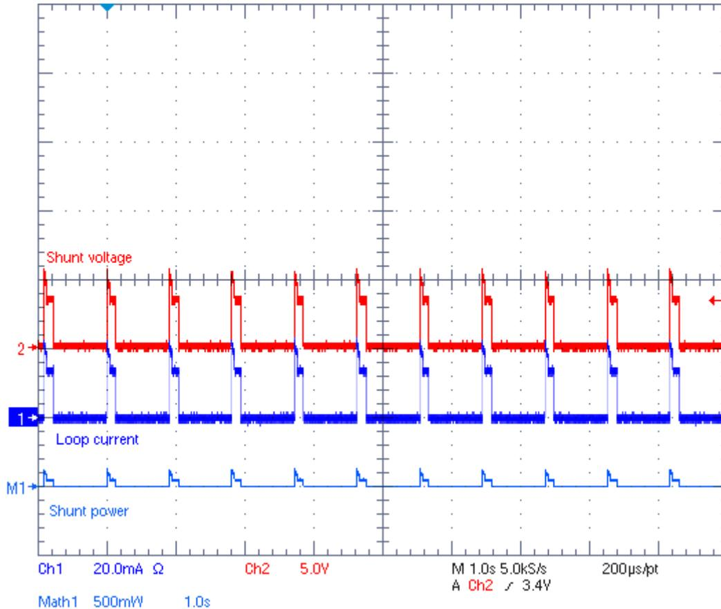
Figure 3-3. TPS26610 Overcurrent Response With  $V_{IN} = 24\text{ V}$  (1 s/div) — 250- $\Omega$  Burden Resistor
