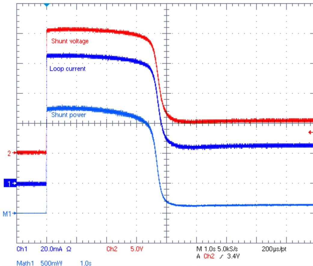
Figure 3-2. PTC Overcurrent Response With  $V_{IN} = 24\text{ V}$  (1 s/div) — 250-Ω Burden Resistor
