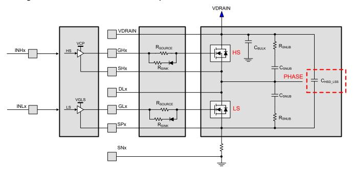
Figure 4-4. Example High-Side Drain to Low-Side Source Capacitor Location
