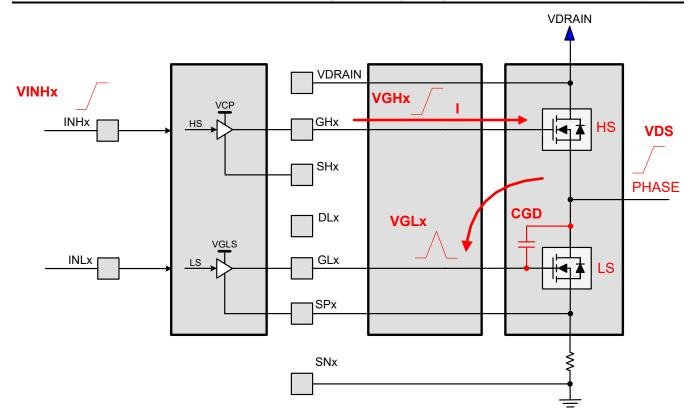
Figure 3-1. Inductive Spiking and Coupling From Switching on MOSFET
