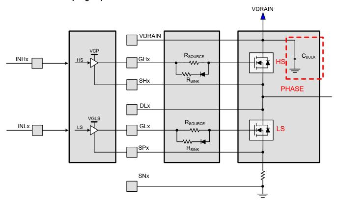
Figure 4-1. Bulk Capacitor Example
