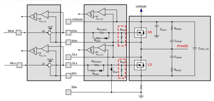
Figure 6-2. Example Passive Gate-to-Source Pulldown Resistors
