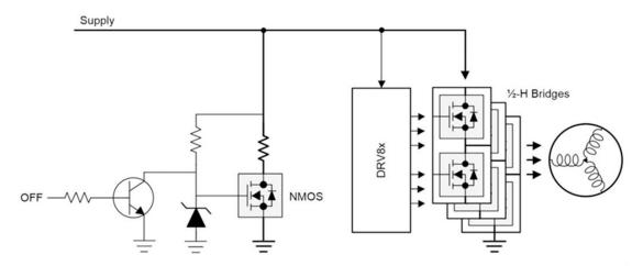
Figure 7-2. Example Active Brake Circuit
