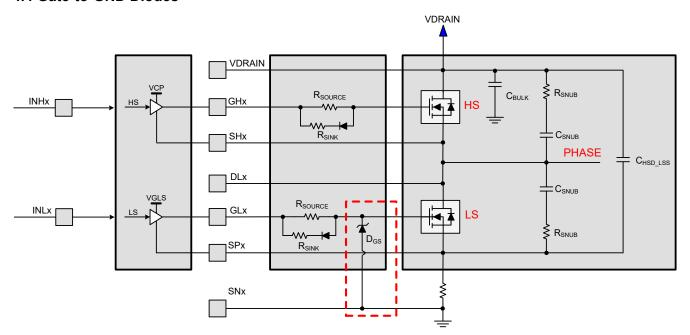
Figure 4-5. Example Gate-to-GND Diode
