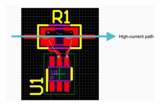
Figure 8-1. Example of a Good Kelvin Connection
