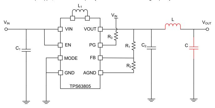
Figure 3-1. TPS63805 Circuit with LC Filter
