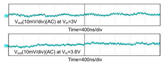
Figure 3-5. Output Voltage Ripple with LC Filter
