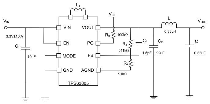
Figure 3-3. Reference Circuit of Voltage Stabilizer
