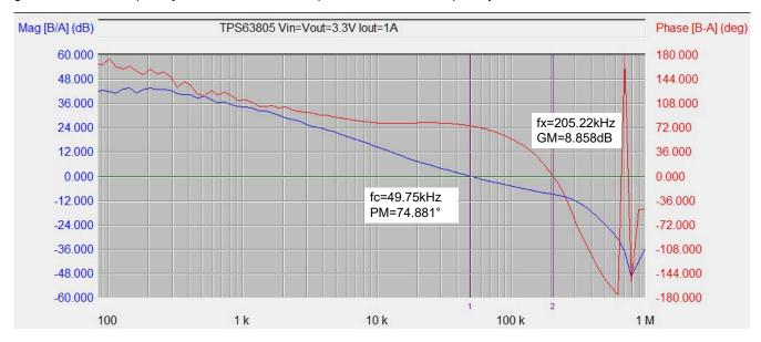
Figure 3-2. Bode Plot of TPS63805 with Default Configuration
