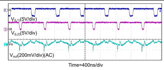
Figure 2-2. Output Ripple Waveforms of TPS63805 at Vin=3.6V, Vout=3.3V, ILoad=0.5A
