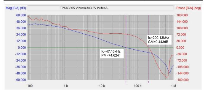
Figure 3-4. Bode Plot of TPS63805 with LC Filter
