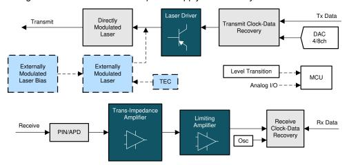
Figure 1-1. Block Diagram of Optical Module
