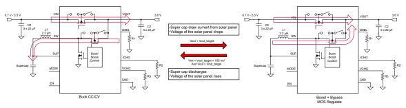
Figure 3-3. Main Two Operation States Transition
