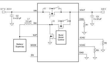
Figure 3-2. Typical Application of TPS61094
