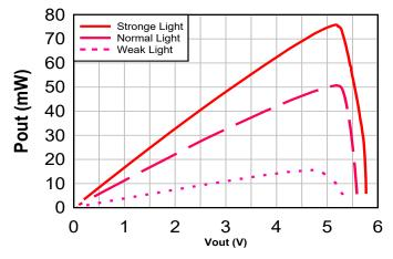
Figure 3-1. V-P Curve of Solar Panels under Different Environment
