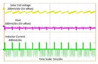
Figure 3-4. Typical Waveform to Realize MPPT
