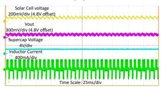
Figure 4-2. Strong Light and 20 mA Load Operation Waveform
