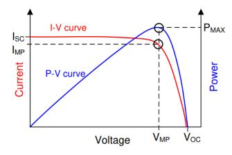
Figure 1-1. VI/VQ Curve of Solar Cell
