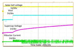
Figure 4-1. The Supercap Charging under Strong Light Conditions
