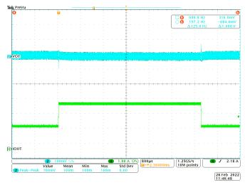
Figure 2-9. TPS563211 AECM Transient Response 1.5A-3A
