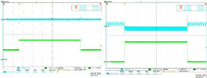
Figure 2-3. Part1 PCM Transient Response 1.5A-3A
