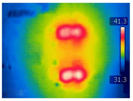
Figure 3-6. Heat Distribution of Dual Converter
