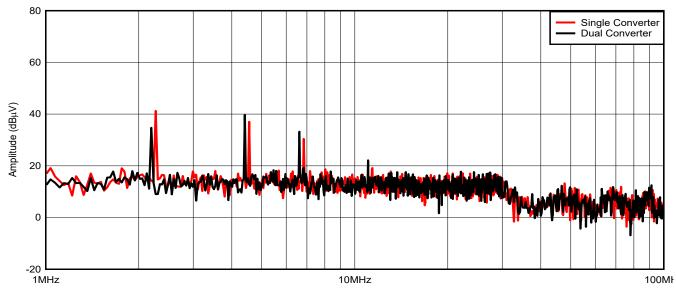
Figure 3-3. Output Voltage Ripple of the Single 5onverter and Dual Converter
