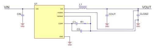
Figure 2-1. Single Converter Schematic
