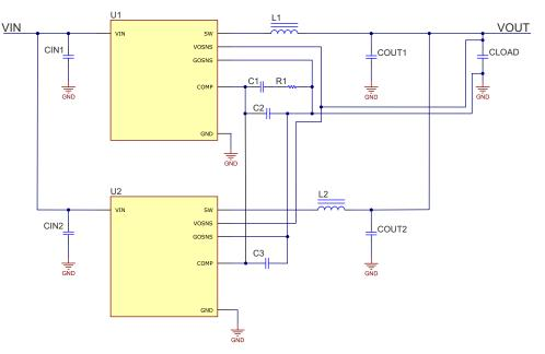
Figure 2-2. Dual Converter Schematic
