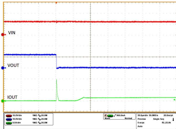
**Figure 8. TPS25961 Short at Output Protection**
