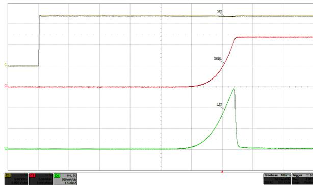
Figure 5. Discrete design Inrush Current Control
