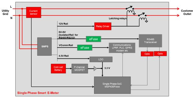
**Figure 6. Single Phase Smart E-meter**
