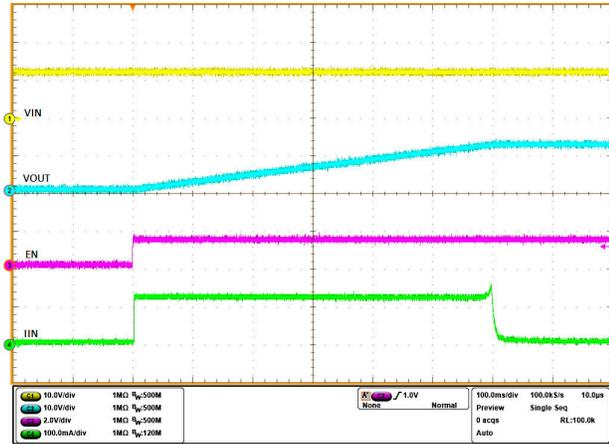
**Figure 7. TPS25961 Charging 6400 uF at 0.1 A Current Limit**
