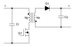
Figure 1. Nonsynchronous Flyback Converter Schematic
