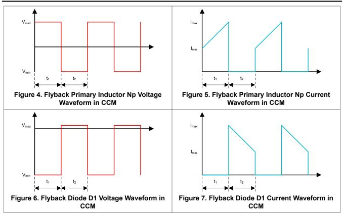
Low-power or low-output-current flyback converters are often designed to operate in discontinuous conduction mode (DCM) to minimize transformer size, weight, and cost. An additional benefit of this approach is that the  $R_{HPZ}$  frequency moves to regions higher than 100 kHz, enabling higher regulation bandwidths than in CCM.
