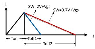
Figure 3-4. Inductor Current with Different AVIN
