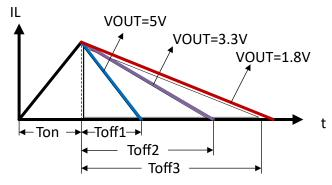
Figure 3-5. Inductor Current for Different VOUT
