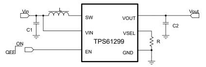
Figure 2-1. Typical Schematic of Traditional Start-up Design
