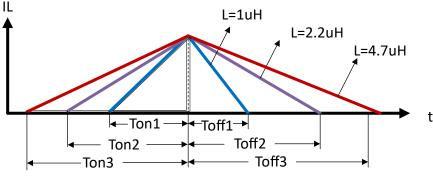
Figure 3-6. Inductor Current With Different L
