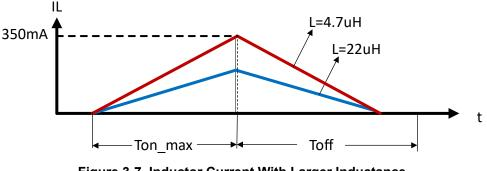
Figure 3-7. Inductor Current With Larger Inductance
