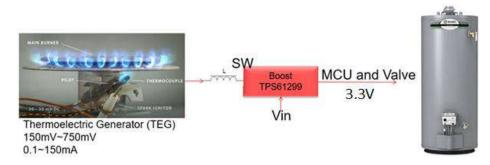
Figure 1-1. Water Heater Control Diagram
