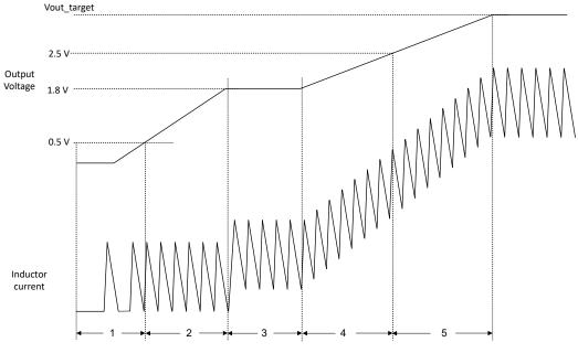
Figure 2-3. Start-up Process of TPS61299
