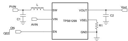
Figure 2-2. Typical Schematic With Ultra Low Input Voltage Start-up Design
