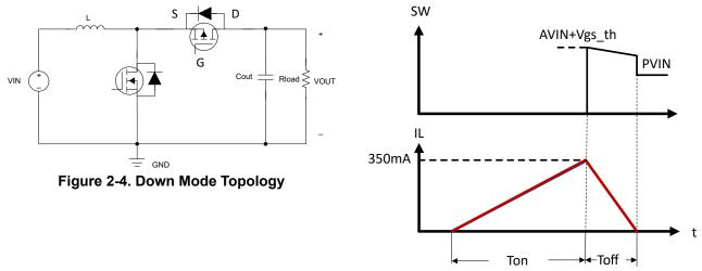
Figure 2-5. Down Mode Waveform
