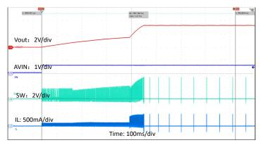
Figure 4-1. 80 mV PVIN Start-up Waveform
