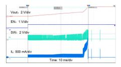
Figure 3-1. TPS61299 150 mV Input Voltage Start-up
