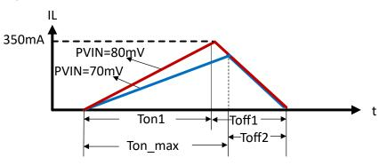
Figure 3-10. Inductor Current Curves for Different PVIN
