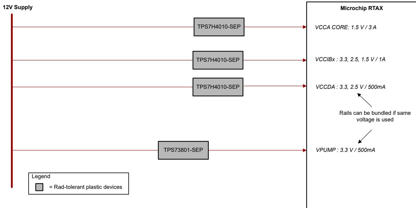
**Figure 4-2. Rad-Tolerant Power for RTAX**
