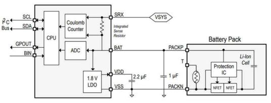
Figure 3-9. BQ27427 Gauge Function Block
