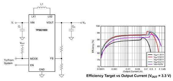
Figure 4-3. TPS631000 Efficiency
