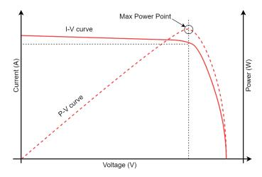
Figure 3-4. Solar Cell PV/IV Curve
