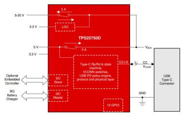
Figure 3-2. TPS25750D Function Block
