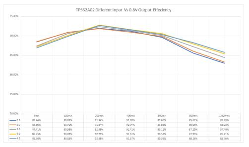
Figure 4-5. TPS62A02 Output 0.8 V Efficiency
