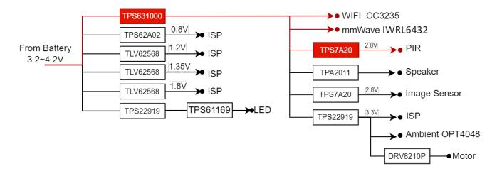
Figure 4-1. Battery Powered Camera Power Tree
