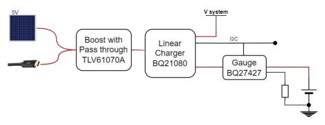
Figure 3-7. Solar Charger Design Function Block
