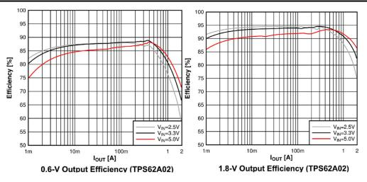
Figure 4-4. TPS62A02 Efficiency
