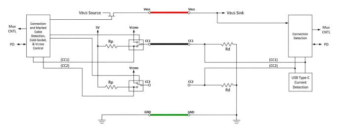
Figure 3-1. USB Type-C Connection Between Source and Sink
