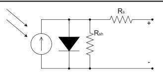
Figure 3-3. Solar Cell Equivalent Circuit
