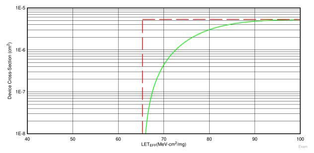
Figure 1-2. Device Cross Section Versus LET<sub>EFF</sub> Showing How the Weibull Fit (Green) is "Simplified" With the Use a Square Approximation (Red Dashed Line)
