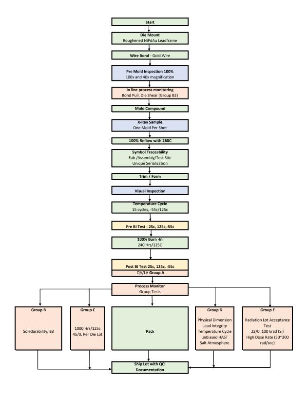
Figure 2-1. TPS7H4001-SHP Space High Grade Plastic Production Flow Chart
