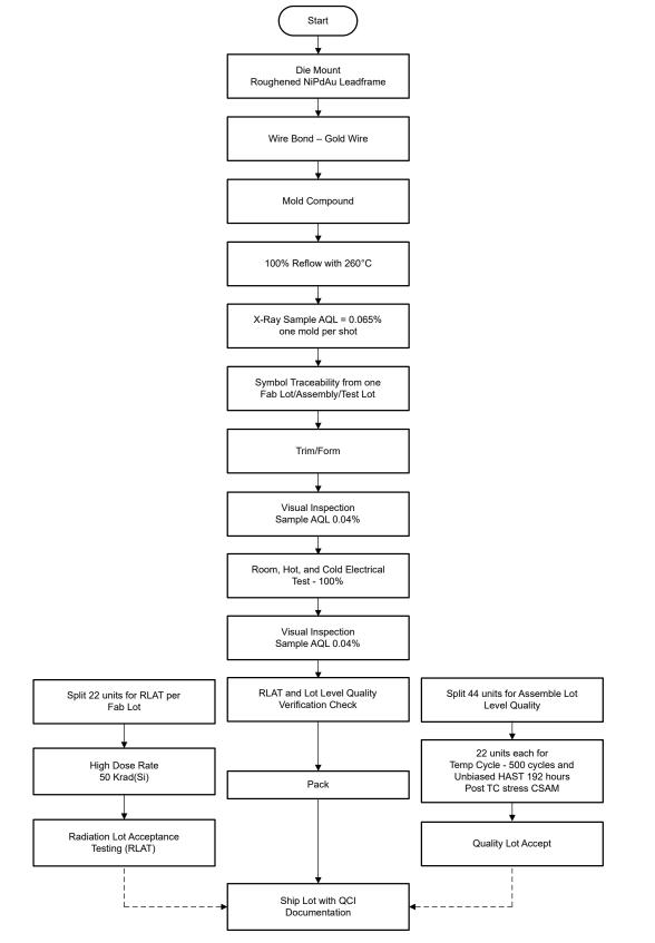
Figure 2-1. TPS7H3302-SEP Space Enhanced Plastic Production Flow Chart
