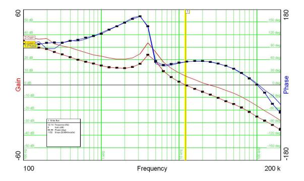
The figure below is the loop gain of the 3.3V converter with max load. The dotted traces are 5V input; the non-dotted traces are 12V input. With a 5V input, the bandwidth is 17 KHz, the phase margin is 56 degrees, and the gain margin is 20 dB. With a 12V input, the bandwidth is 32 KHz, the phase margin is 45 degrees, and the gain margin is 14 dB.
