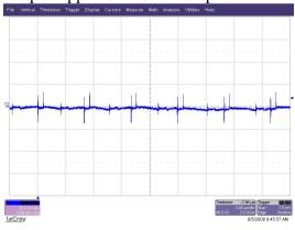
Output ripple/noise 1.2V output:
