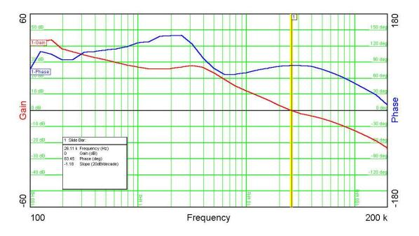
The figure below is the loop gain of the 1.8V converter with max load. The dotted traces are 5V input; the non-dotted traces are 12V input. With a 5V input, the bandwidth is 12 KHz, the phase margin is 55 degrees, and the gain margin is 25 dB. With a 12V input, the bandwidth is 25 KHz, the phase margin is 55 degrees, and the gain margin is 17 dB.
