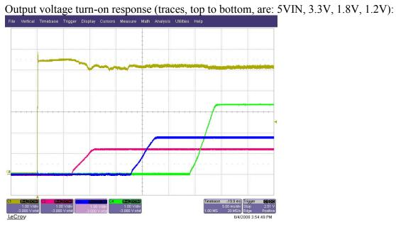
Output voltage turn-on response (traces, top to bottom, are: 12VIN, 3.3V, 1.8V, 1.2V):
