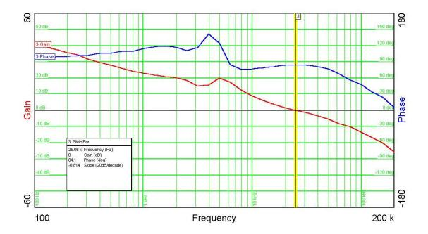
The figure below is the loop gain of the 1.2V converter with a 12V input and max load. The bandwidth is 26 KHz, the phase margin is 83 degrees, and the gain margin is 23 dB.
