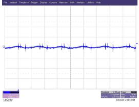
Output ripple/noise 1.8V output:
