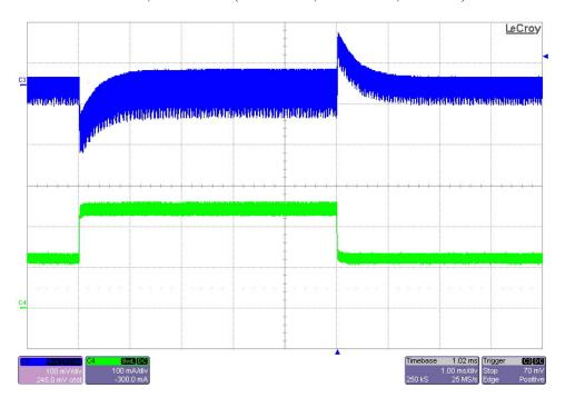
The photo below shows the 6V output voltage (top, ac coupled) when the load current is stepped between 0.125A to 0.25A. Vin = 48Vdc, 8V @ 0.25A (100mV/DIV, 100mA/DIV, 1mS/DIV)
