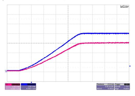
The photo below shows the 8V and 6V output voltage startup waveforms after the application of 48Vdc in. The outputs were loaded to 0.25A each. (2V/DIV, 5mS/DIV)
