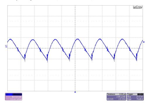
The 6V output ripple voltage is shown in the figure below. The image was taken with both output loaded to 0.25A and the input voltage set to 48Vdc. (50mV/DIV, 2uS/DIV)
