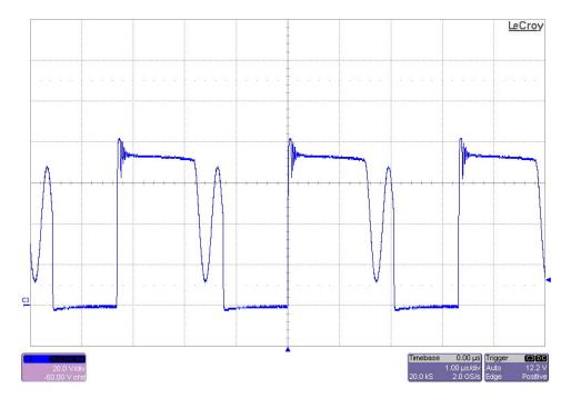
The photo below is of the N-ch FET drain waveform. The input voltage is 60V and the outputs are loaded to 0.05A each. (20V/DIV, 1uS/DIV)
