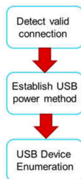
Figure 10-13. Flow of DFP-to-UFP Configuration
