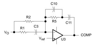
The first step in the design of the error-amplifier frequency response is the design of the output sense divider. This sets the output voltage, and the top resistor, R2, determines the relative impedance of the rest of the compensation design. A 2.32 k $\Omega$  resistor for the top of the divider gives a divider current of 0.99 mA for an output setting of 3.3 V. The bottom of the divider (omitted from Figure 2–3 for clarity) is calculated as:
