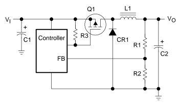
The SLVP101, SLVP102, and SLVP103 buck converters use the Texas Instruments TL5001 PWM controller to give power supply outputs of 3.3 V, 2.5 V, and 1.8 V at 0 to 3 A. Also featured in this design are the TL1431 reference IC, the TPS2817 MOSFET driver IC, and the TLV2231 operational amplifier. These converters operate over an input voltage range of 4.5 V to 9 V with typical efficiences of 90 percent for 3.3 V out and 80 percent for 1.8 V out.
