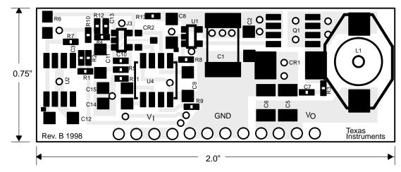
Figure 1–4. Component Placement Showing Component-Side Copper
