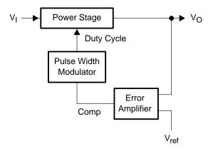
The following is a simplified approach to designing networks to stabilize continuous mode buck converters. It works well when the open-loop gain is below unity at a frequency less than one-half of the switching frequency of the power supply.
