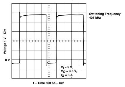
Figure 1–15. SLVP101 (3.3 V Output) TL5001 PWM Output Switching Waveform
