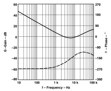
The overall open loop frequency response of the converter is the product of the uncompensated open loop response (Figure 2–2) and the error amplifier response (Figure 2–4). A Bode plot of the overall open loop frequency response of the converter is shown in Figure 2–5. Again, the solid line is the gain and the dashed line is the phase. As seen in the graph, the gain crosses 0 dB in the vicinity of 20 kHz and the phase margin is approximately 100 degrees.
