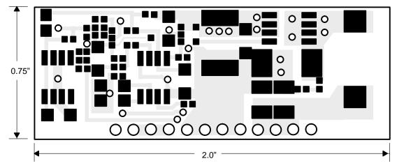
Figure 1–6. Solder-Side Copper
