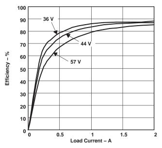
Figure 4. Typical 5-V DC/DC Converter Efficiency
