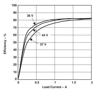
Figure 3. Typical 5-V PD End-to-End Efficiency
