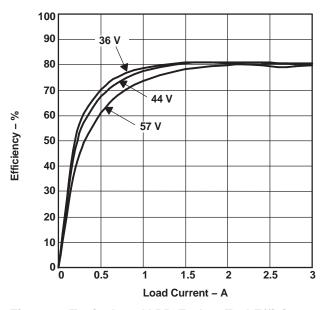
Figure 1. Typical 3.3-V PD End-to-End Efficiency
