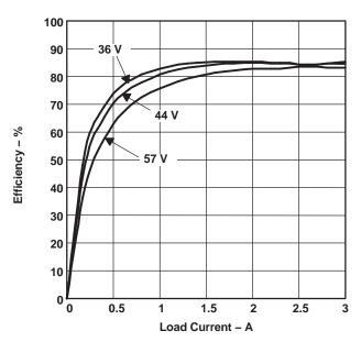
Figure 2. Typical 3.3-V DC/DC Converter Efficiency
